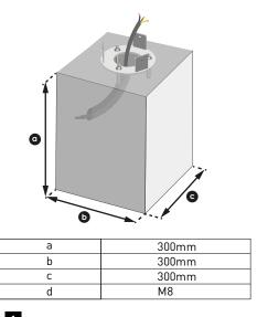
1 1 steel flange required during assembly is available as mounted on the product. Steel dowel (3xM8) must be provided by the assembly team.
