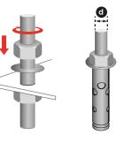
2 After flange set on the surface, mark the steel dowel holes. Drill the steel dowel holes with a suitable drill. Then place the steel dowels without nuts on the flange surface. Use the nuts to fix flange into the concrete ground. Next step will be the connection of cables.
