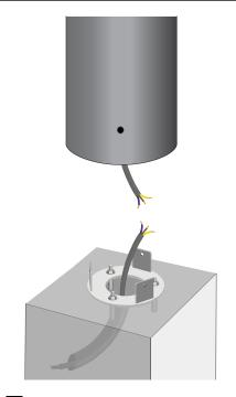
Please use the electrical connection table to connect cables. Be sure that earthing connection has done.
