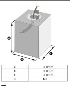
1 steel flange required during assembly is available as mounted on the product. Steel dowel (3xM8) must be provided by the assembly team.
