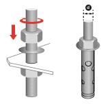
After flange set on the surface, mark the steel dowel holes. Drill the steel dowel holes with a suitable drill. Then place the steel dowels without nuts on the flange surface. Use the nuts to fix flange into the concrete ground. Next step will be the connection of cables.
