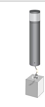
After cable connection, mount the product to the flange with 3 nos screws.
