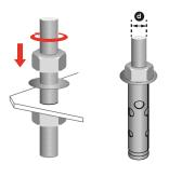
After flange set on the surface, mark the steel dowel holes. Drill the steel dowel holes with a suitable drill. Then place the steel dowels without nuts on the flange surface. Use the nuts to fix flange into the concrete ground. Next step will be the connection of cables.
