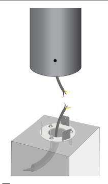
Please use the electrical connection table to connect cables. Be sure that earthing connection has done.
