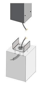
Please use the electrical connection table to connect cables. Be sure that earthing connection has done.
