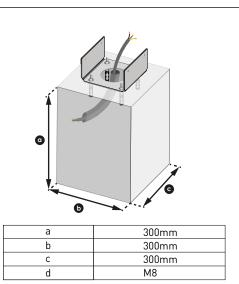
1 Steel flange required during assembly is available as mounted on the product. Steel dowel (4xM8) must be provided by the assembly team.
