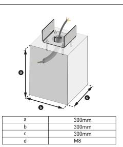
1 steel flange required during assembly is available as mounted on the product. Steel dowel (4xM8) must be provided by the assembly team.
