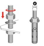
2 After flange set on the surface, mark the steel dowel holes. Drill the steel dowel holes with a suitable drill. Then place the steel dowels without nuts on the flange surface. Use the nuts to fix flange into the concrete ground. Next step will be the connection of cables.
