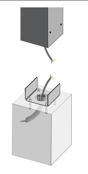
Please use the electrical connection table to connect cables. Be sure that earthing connection has done.
