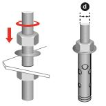
2 After flange set on the surface, mark the steel dowel holes. Drill the steel dowel holes with a suitable drill. Then place the steel dowels without nuts on the flange surface. Use the nuts to fix flange into the concrete ground. Next step will be the connection of cables.
