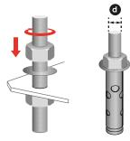
After flange set on the surface, mark the steel dowel holes. Drill the steel dowel holes with a suitable drill. Then place the steel dowels without nuts on the flange surface. Use the nuts to fix flange into the concrete ground. Next step will be the connection of cables.
