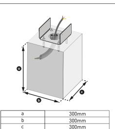
1 steel flange required during assembly is available as mounted on the product. Steel dowel (4xM8) must be provided by the assembly team.
