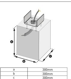
d M8 **1** 1 steel flange required during assembly is available as mounted on the product. Steel
